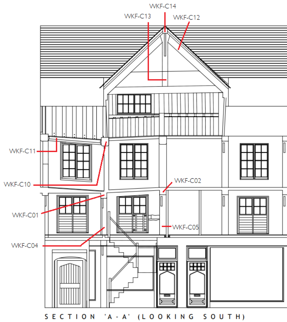
Figure 5: Section, showing sampled timbers. [inc. architecture limited]
