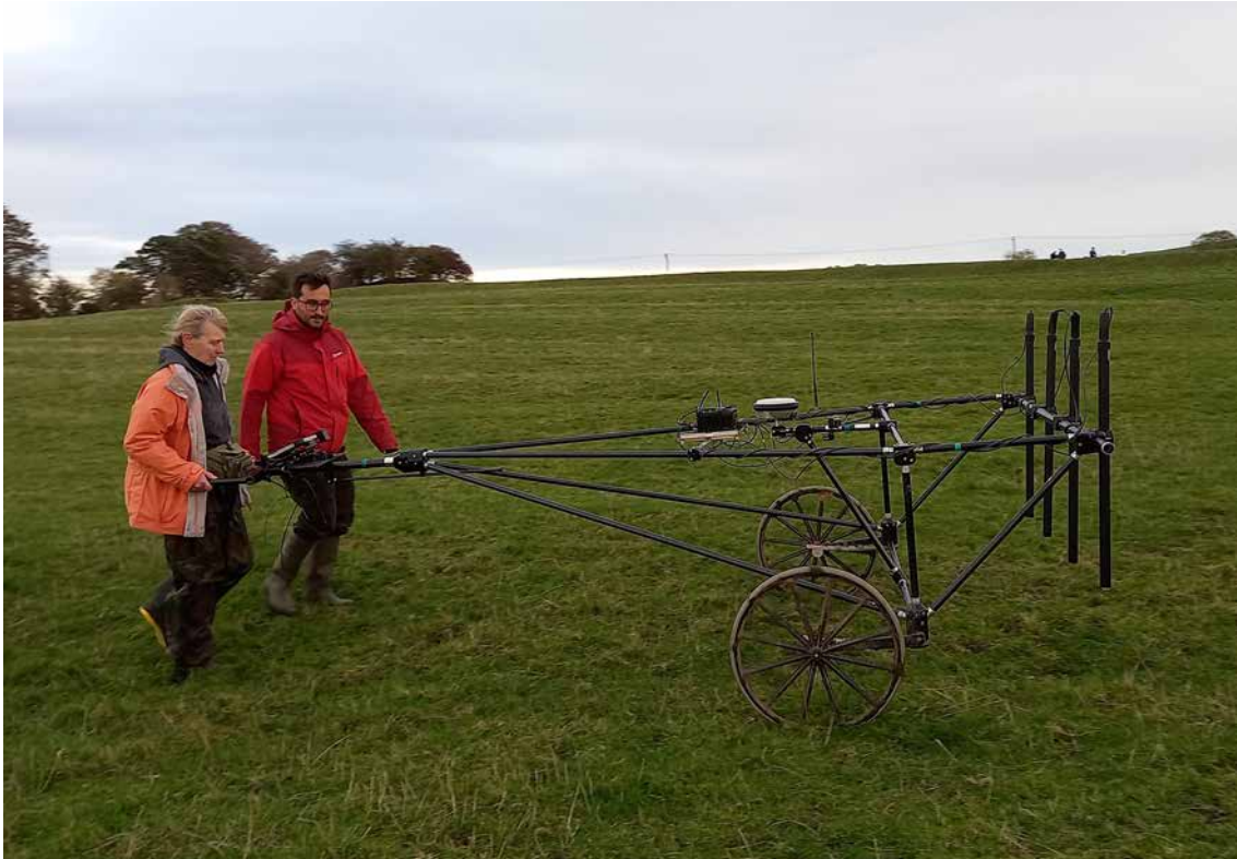
Figure 33: Wessex Archaeology's cart-mounted gradiometer in use at Chester Crane Camp, November 2022. [© Historic England]
