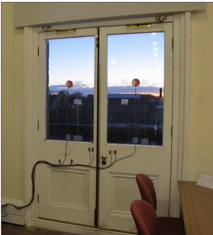
Figure 14: In-situ U-value measurements of the double glazing system. Heat flux and surface temperature sensors are attached to the acrylic panes.
