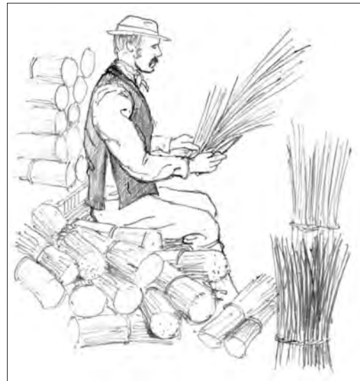
Figure 5. Trimming straws by hand.
