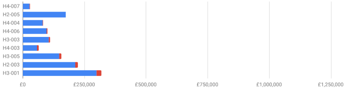
Figure 29 – Cumulative Cost of Delayed Repair – 9 churches with regular maintenance/repair
