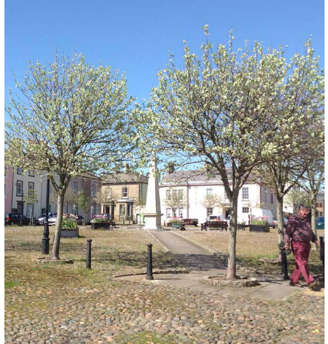
Fleming Square, Maryport, Cumbria. This traditional pebble stone paving provides a beautiful and durable surface. If possible, smooth paving can be provided to assist users of wheelchairs or buggies.
