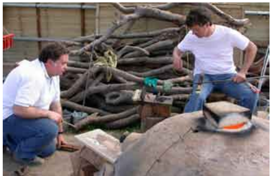
The Roman Glassmakers: Mark works the glass (right) with the assistance of David (left). A partly formed glass vessel is on the end of the blowing iron, which Mark supports on wooden thigh-boards. A selection of glassworking tools are to hand and fuel is piled in the background ready for use
