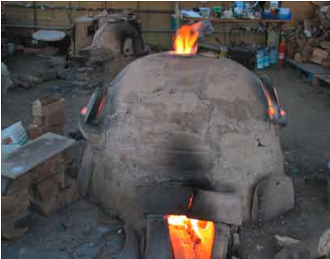
The pot furnace at dusk, with flames being drawn into the stoke hole at the front, gathering holes to the left and right (and another at the rear) and a small vent in the top of the domed roof. Behind the pot furnace can be seen the second smaller experimental furnace with an adjoining oven for annealing the glass
