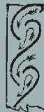
Section of Acme Patent Curved Exhaust Louvres. The arrows show the action of the wind and exhaust.
