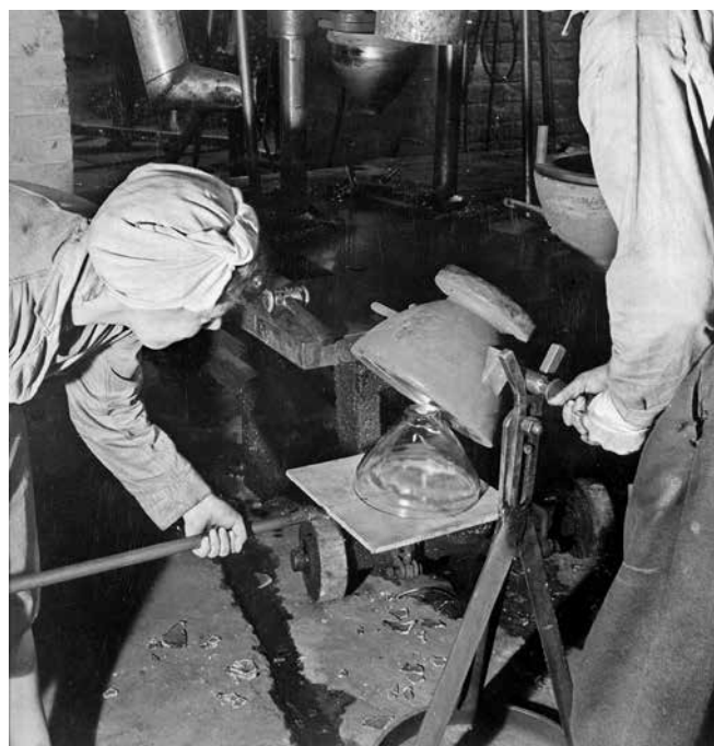
Figure 46 Removing the glass cone for a cathode ray tube from a hand press, comprising a plunger and mould, at Osram glassworks, Newcastle upon Tyne, Tyneside, in the mid-20th century.
