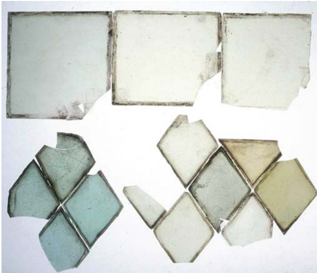
Figure 62 The characteristic colours of post-medieval window glass, from green (high-lime low-alkali; HLLA), to pale blue (kelp) to colourless (synthetic soda).
