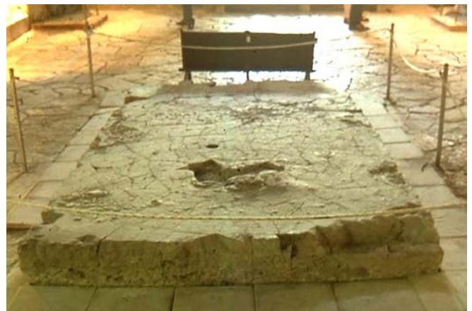
Figure CS3-2 (right) A slab of failed glass made in a tank furnace from Bet She'arim, Israel. The slab is circa 2m wide and weighs circa 9 tonnes. Analysis suggests that it dates to around the 9th century.
