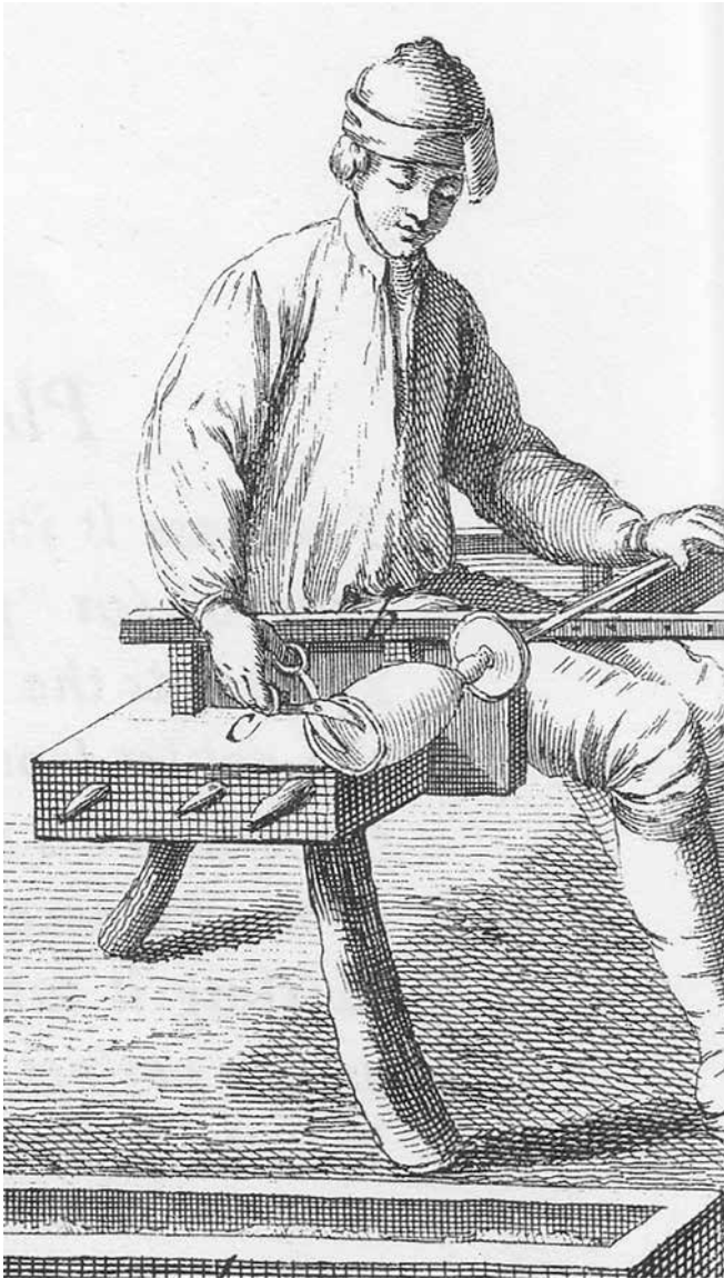
Figure 43 (left) Formation of wavy ribbons in a mid-18th-century illustration of goblet production by Diderot.
