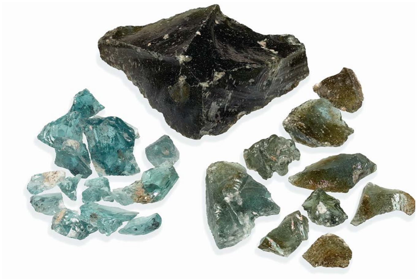
Figure 31 Fragments of raw Roman soda-lime-silica natron glass excavated at Basinghall Street, London; the width of the top fragment is 128mm.
