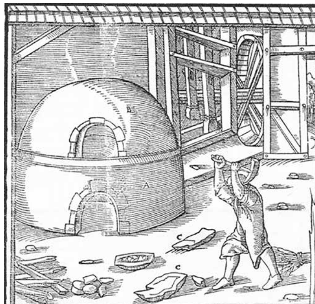
Figure 8 16th-century depiction of fritting from Agricola; the batch was fritted in the upper furnace section, then broken up and melted.
