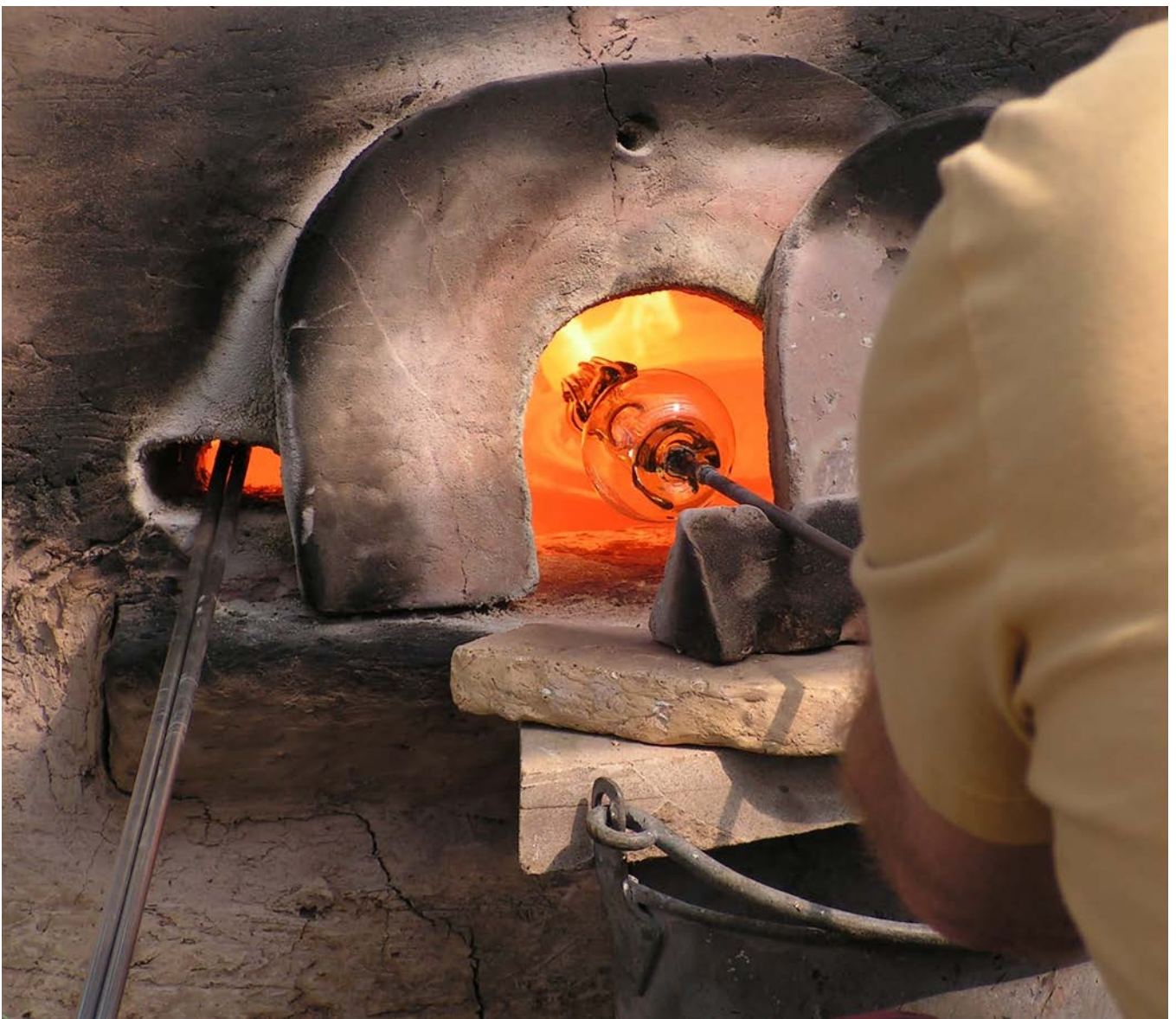
Figure 1 Glassworker reheating an object in a replica Roman furnace made by Mark Taylor and David Hill.
