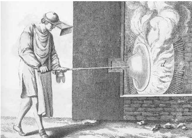
Figure 47 (top) Broad glass production shown in a mid-18th-century illustration by Diderot.
