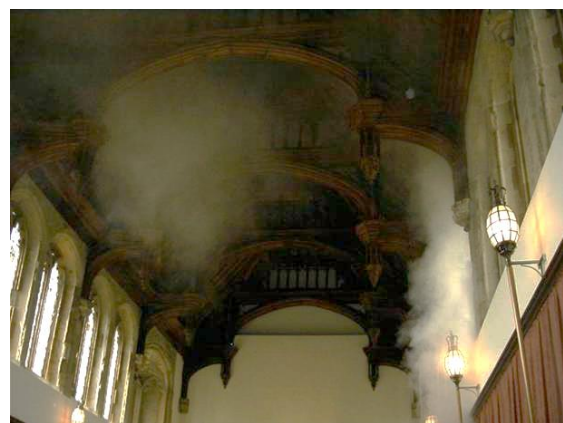
Smoke rising in a convection current and then falling as it cools.
