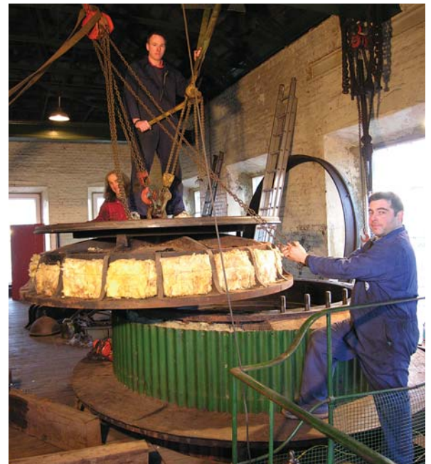
Volunteers removing the cylinder head of the 70-inch Bull engine built by Harvey's of Hayle. The restoration of this engine to working order received the Institution of Mechanical Engineers' Engineering Heritage Award and the Association for Industrial Archaeology's Dorothea Award for Conservation. © Kew Bridge Steam Museum
