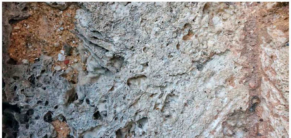
Figure 38: Church of St Ippolyts, St Ippolyts. Detail of tufa, showing porous structure.
