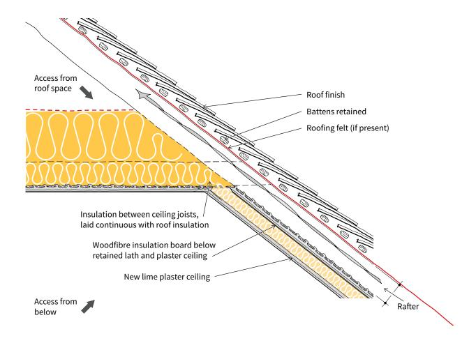
Figure 5: Insulating short sloping ceilings from above. (Rigid insulation pushed down from roof space.) It may be possible to access short sloping ceilings from the open roof space above. If this is the case, rigid batts of insulation can be pushed down into place between the ceiling and roof finish. © Historic England
